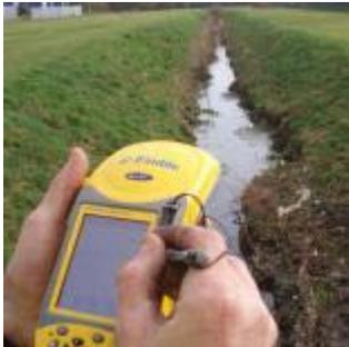
This can help to establish upstream or downstream connectivity of a drainage system to resolve connectivity related issues or can be carried out in conjunction with GPS equipment to fix the location of a pipeline through a site for reasons such as re-development, land registry issues and disputes regarding drainage routes etc. This equipment has also been effectively deployed on road gully connectivity investigation surveys to establish discharge point.
